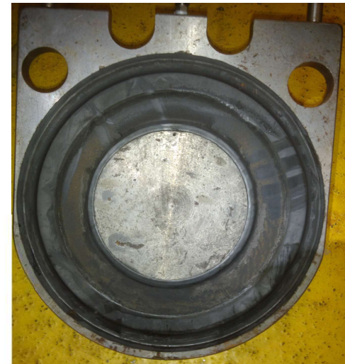
Spade removed after end operation
